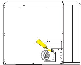
**Step 4.** Install silicone around connection between co-axial adaptor and co-axial air-inlet duct.
